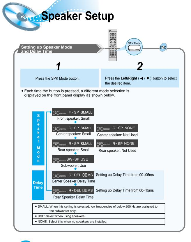
The display changes depending on the current audio output mode (DSP, PRO LOGIC, 3-STEREO, STEREO, etc.).
